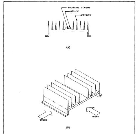
fig. 3. (A) Large finned heatsink used with TO-3 transistors, high-current voltage regulators, high current diodes and SCRs. (B) The "right" and "wrong" way of forcing air over finned surfaces.
